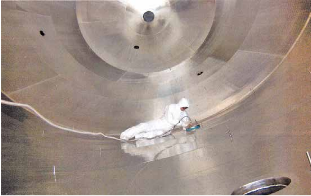
Figure 3: Testing a welded seam at the transition between the main vessel and a socket.
